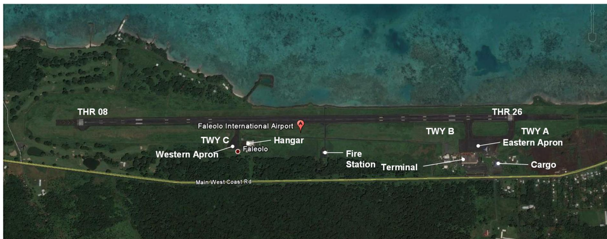
Figure 2 APW general existing airport layout (Source: Aerial photography from Google Earth Pro, dated 4 January 2015.)
