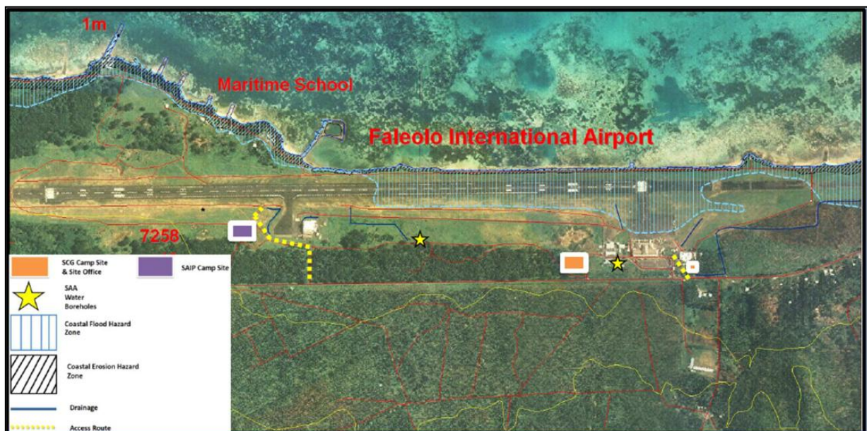
Figure 8 The potential coastal flood hazard at the Faleolo International Airport (APW) (Source: CB Group, 2015.)
